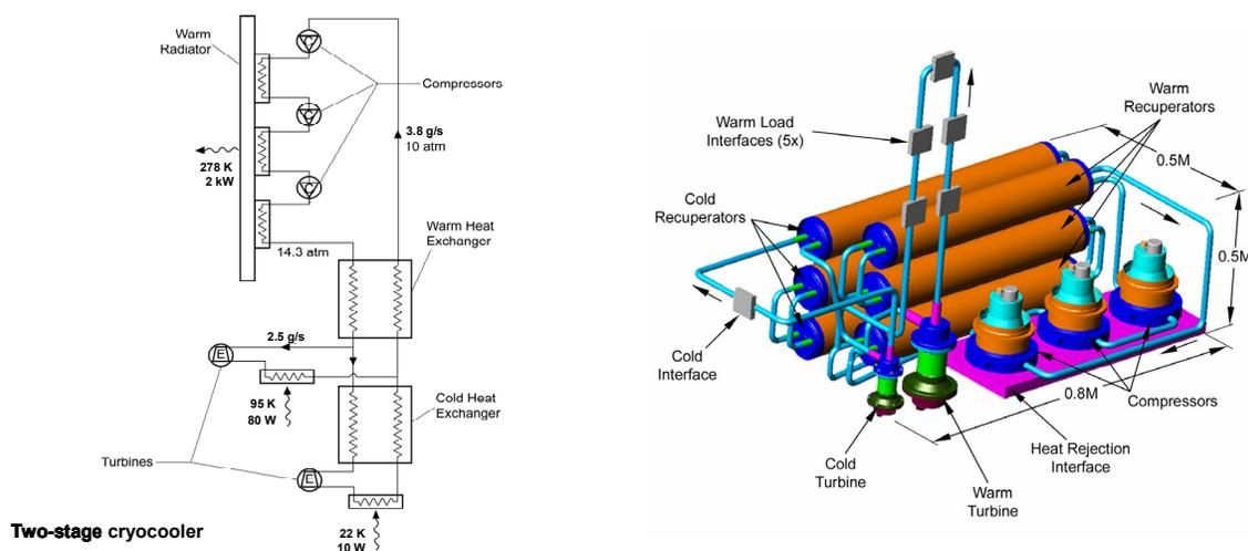
Figure 3-1. ACES Cryocooler Configuration and Layout
