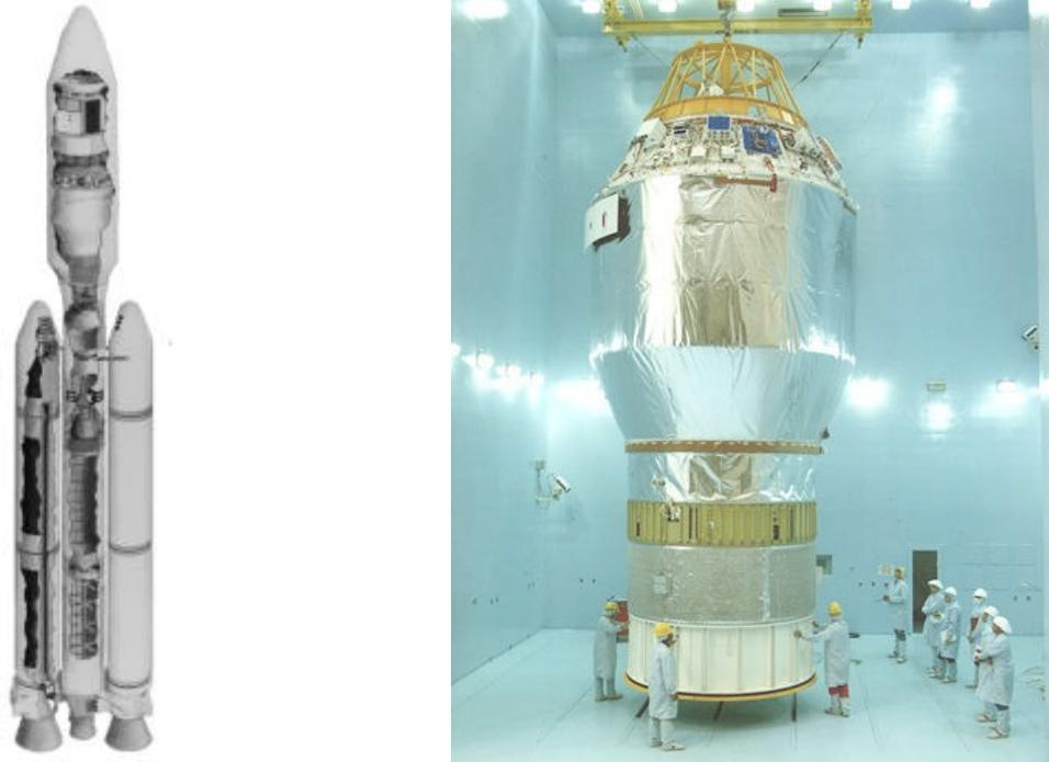
**Figure E. Titan IVB Centaur Launch Vehicle Configuration**
