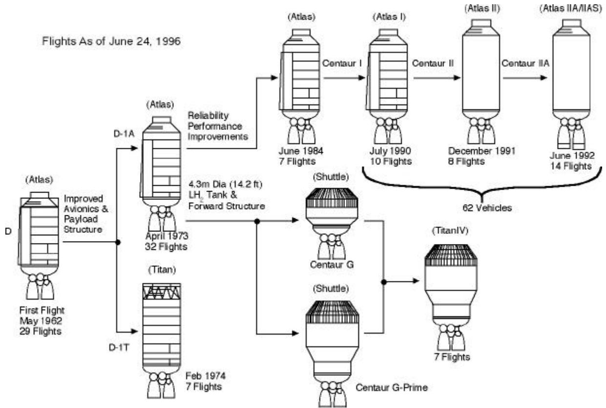
**Figure B. Evolution of the Centaur Upper Stage from the Atlas Centaur to the Titan IV Launch Vehicle**
