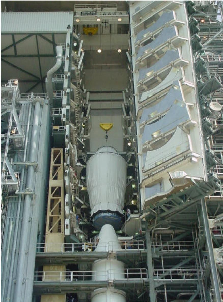
**Figure K. Titan Centaur TC-23 being installed on the Core Vehicle TIVB-35 at LC-40**
