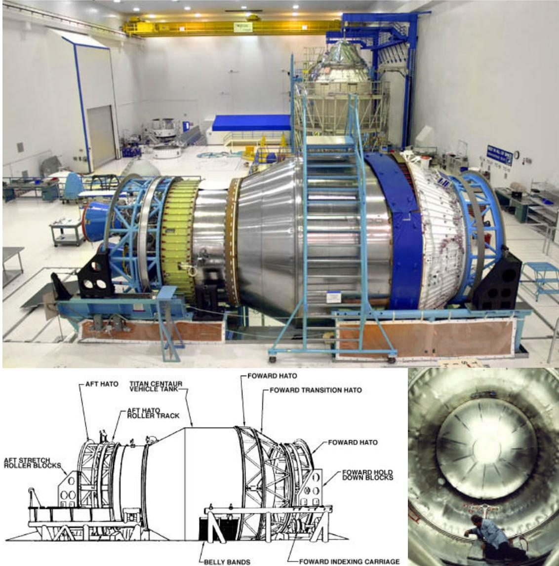
**Figure G. Titan IV Centaur Large Diameter Hydrogen Tank During Manufacture**
