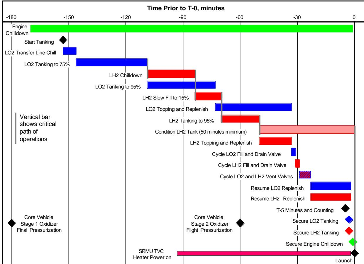
**Figure L. Titan/Centaur Cryogenic Launch Countdown Operations Timeline**
