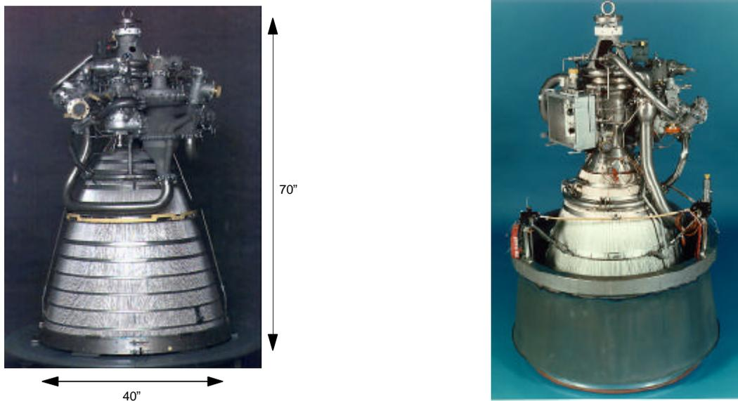
**Figure I. TIV Centaur Pratt & Whitney Engines, RL10A-3-3A (left) & RL10A-4-1 (right)**
