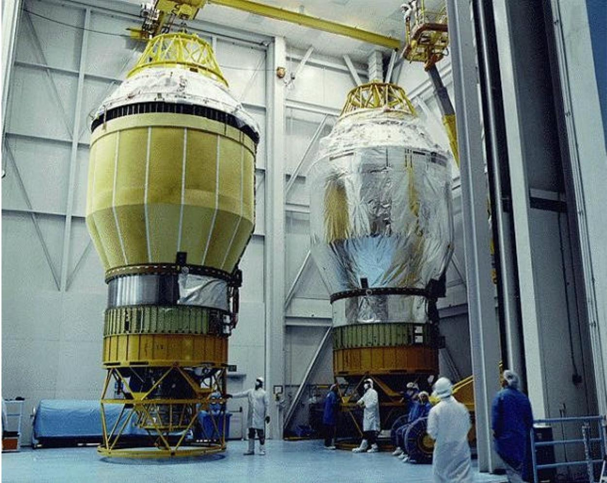
**Figure H. Titan Centaur in the Thermal Acoustic Facility in San Diego**
