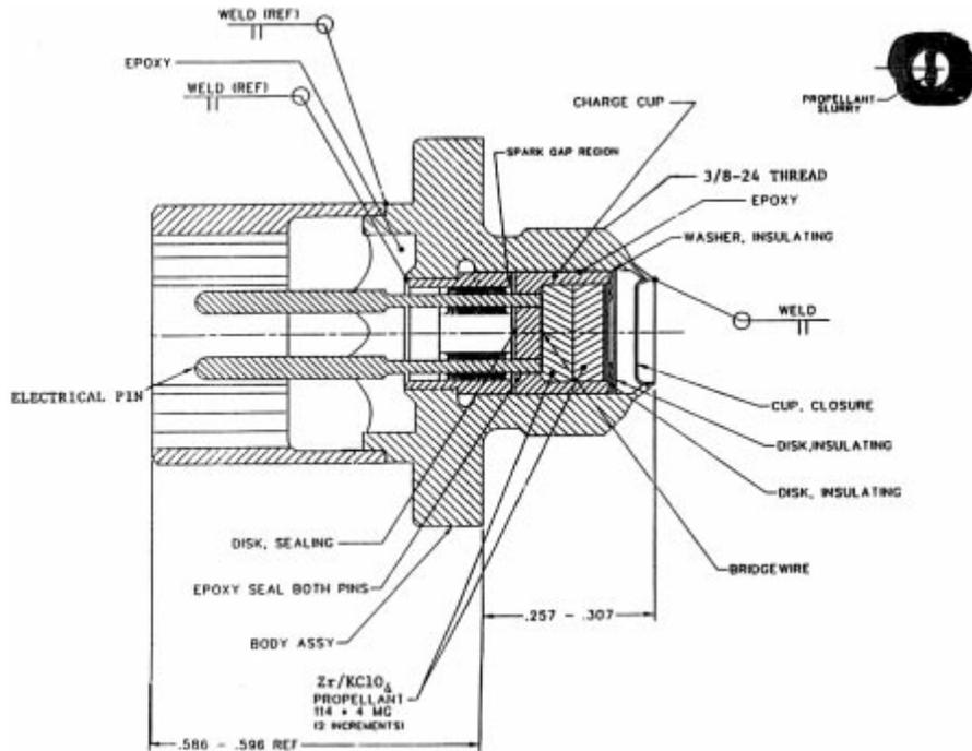
Figure 5 – Cross sectional view of NASA Standard Initiator (NSI)
