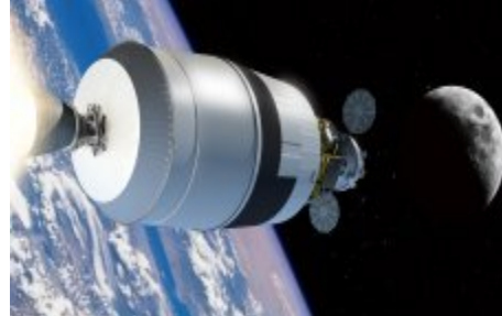
Figure 4 – Concept image of the Ares V EDS in orbit, shown with Orion docked with the Lunar Lander. (Credit: NASA)
