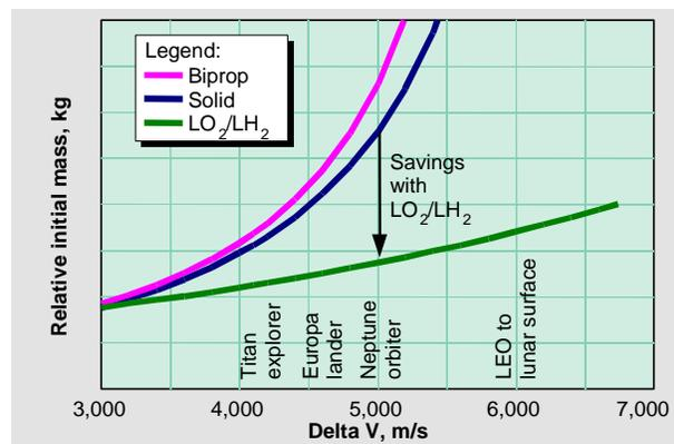
Figure-1, Relative Propellant Performance
