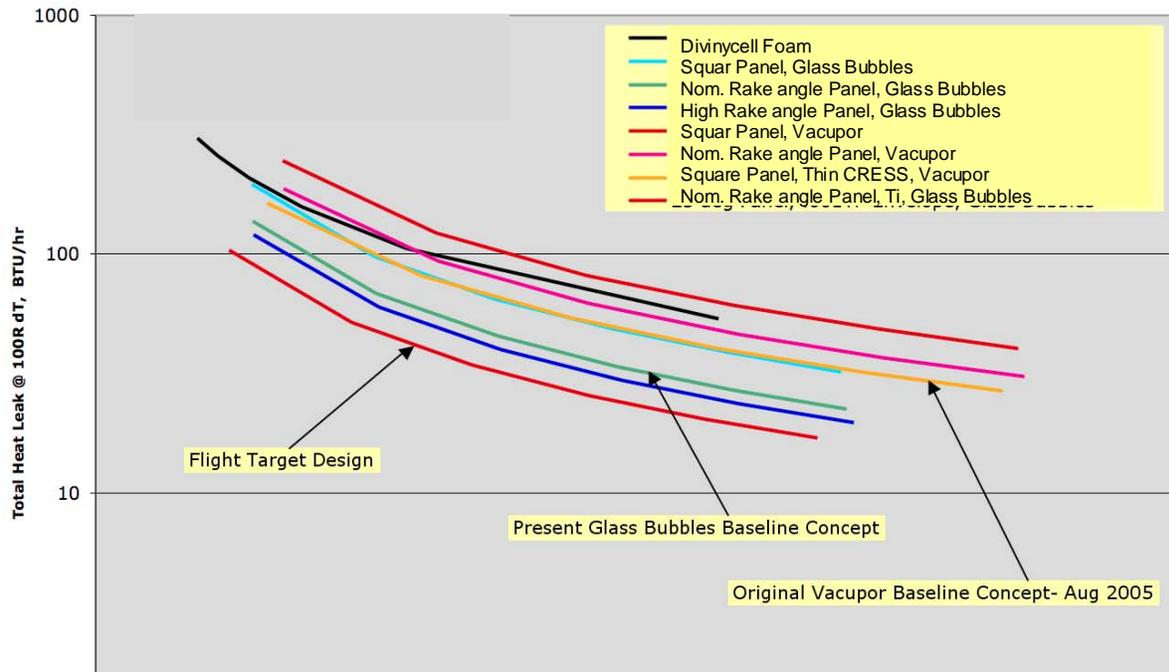
**Figure 5, Vacuum Insulation Panel Materials**
