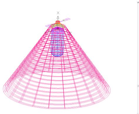
**Figure 8. The thermal analysis accounts for the major heat sources, Solar, Earth and avionics and the radiative and conductive flow paths through the depot. Credit NASA**
