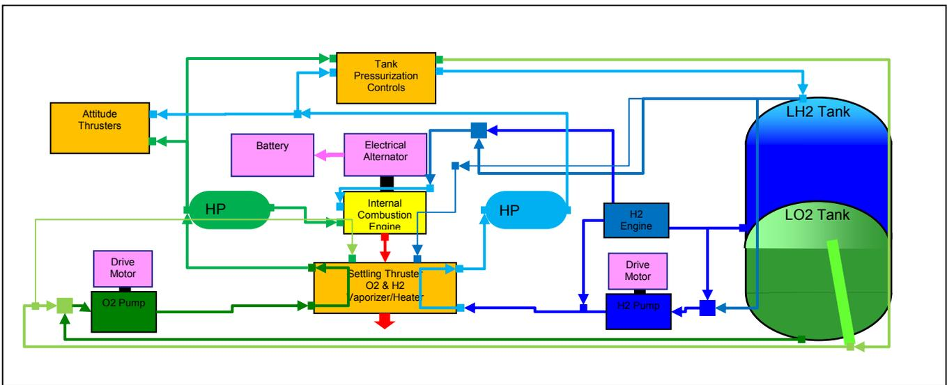
Figure 1: Integrated Vehicle Fluids (IVF) Schematic
