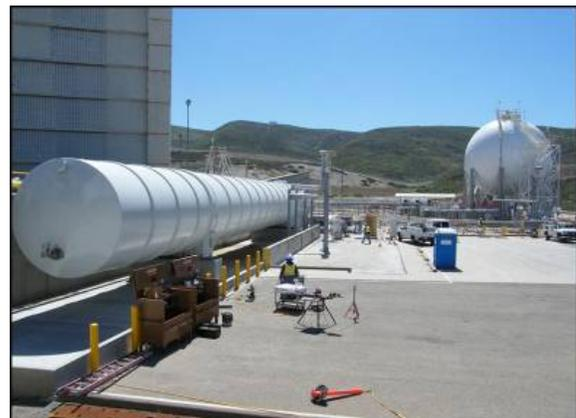
Fig. 10: The Cylindrical Auxiliary LOX Tank in Position
