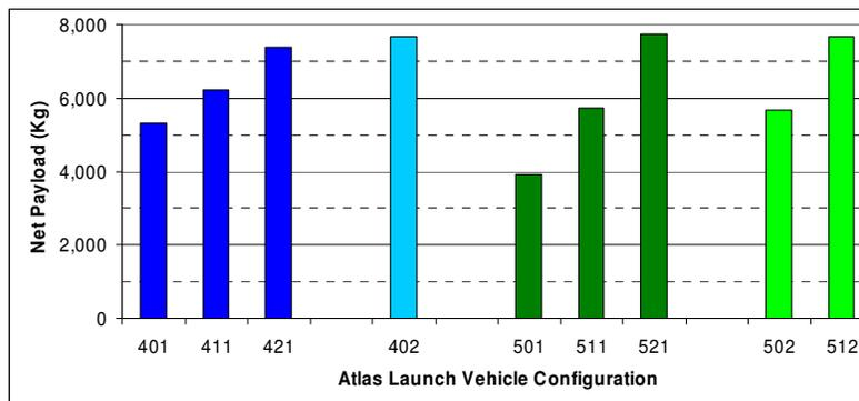
**Figure 11. ARCTUS can take advantage of the modularity of the Atlas launch vehicle to support the customer required payload mass**
