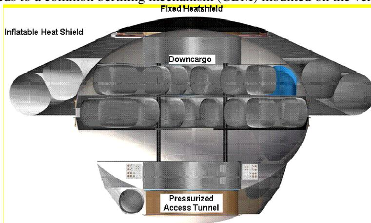
**Figure 8. ARCTUS Pressurized Cargo Accommodations provide 400 ft<sup>3</sup> of conditioned payload volume supporting both up and down mass.**
