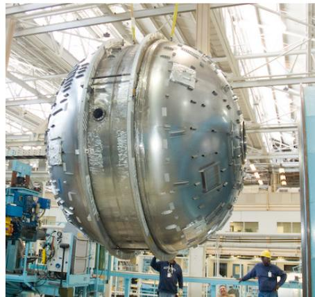
**Figure 5. The ARCTUS Pressurized Reentry Module is built from 2 Centaur domes.**
