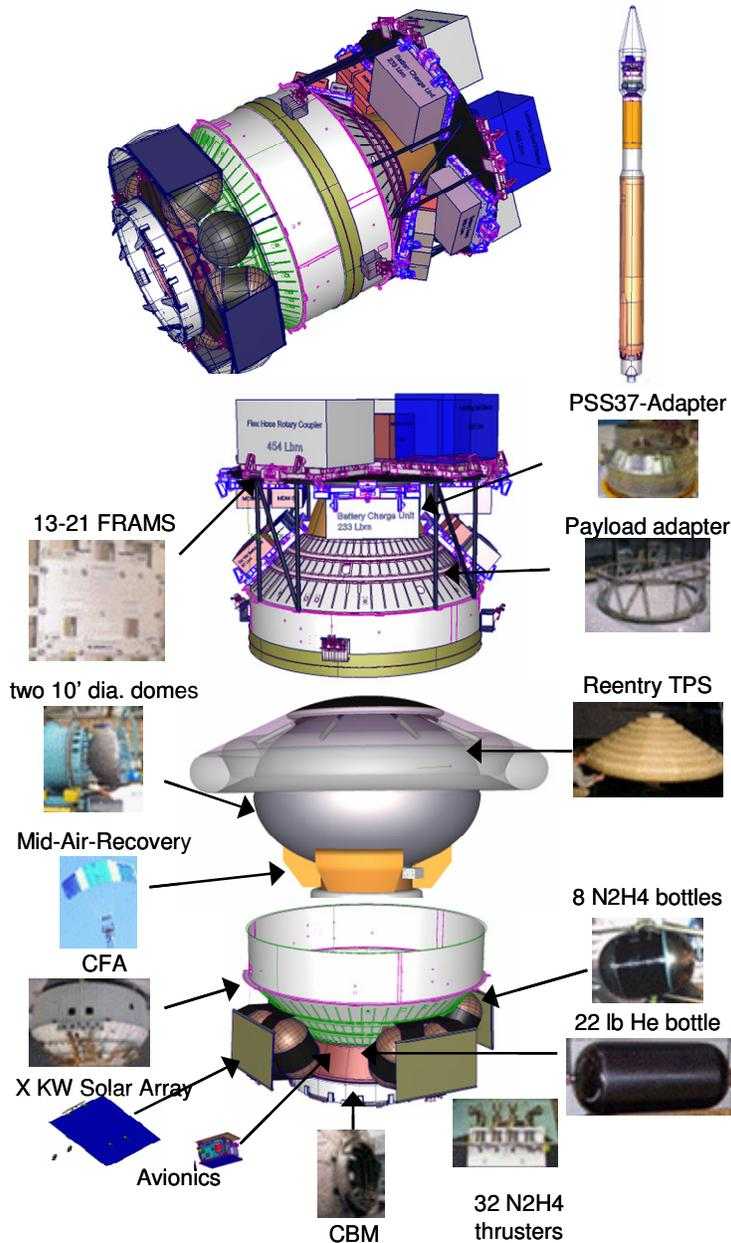
**Figure 2. ARCTUS is primarily derived from existing, flight qualified components that are currently in production**
