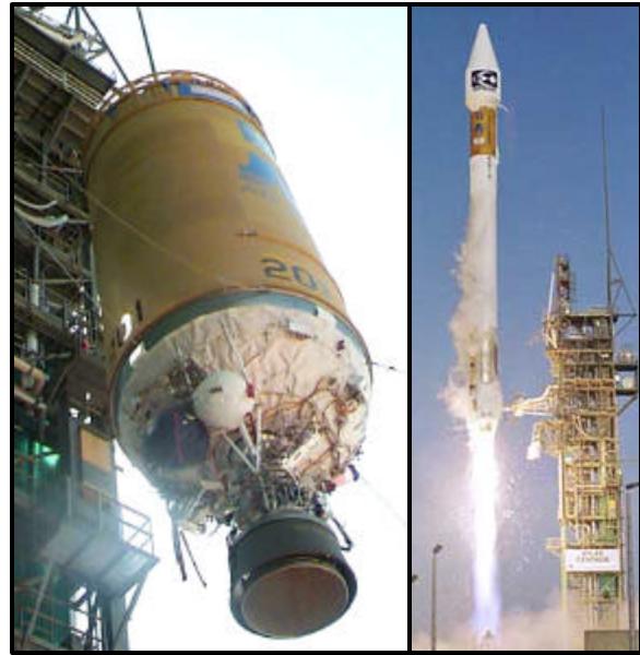
Left: The first Single Engine Centaur is hoisted into position for booster mating at the launch site. Right: The first Atlas IIIA successfully lifts off the launch pad in May 2000.
