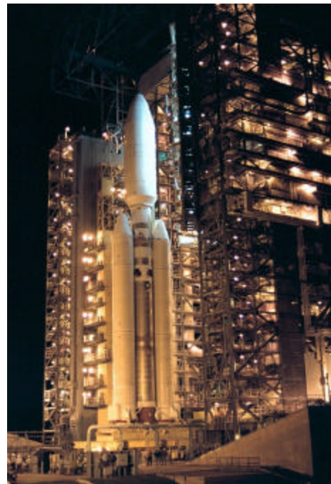
Titan Centaur launch vehicle in the tower with Cassini mission (NASA photo)
