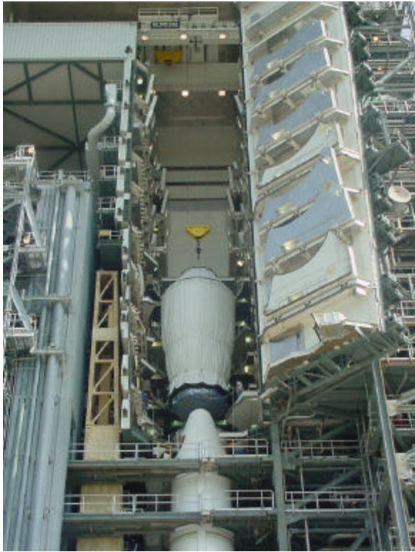
Titan Centaur erection on Titan vehicle at the launch pad
