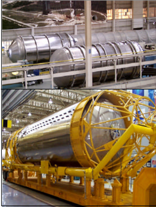
Upper: A Common Centaur tank is shown in San Diego below a Centaur II tank. Lower: A Common Centaur tank leaves San Diego bound for final assembly in Denver.
