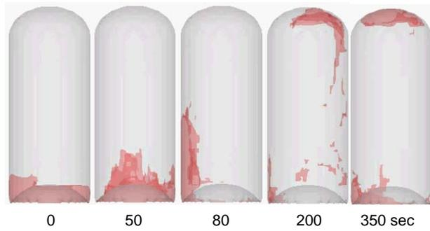
**Figure 3 The Use of Reverse Settling and Transverse Spin Will Reorient the LH2 to the Forward End of Centaur’s LH2 Tank Enabling Bubble Free Liquid Acquisition.**
