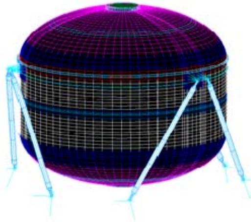
Figure 6 - Ball Aerospace flight heritage cryogenic strut technology has been optimized to meet the structural and thermal requirements of the CRYOTE missions
