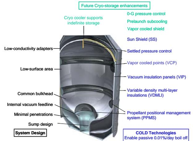
**Figure 4. A combination of upfront tank design and cryogenic fluid storage technologies enable efficient passive LO<sub>2</sub>/LH<sub>2</sub> storage supporting long duration missions.**
