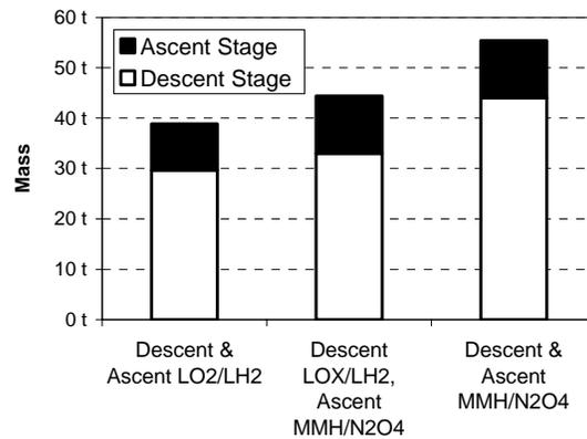
**Figure 1. The use of LO<sub>2</sub>/LH<sub>2</sub> propulsion for the lander reduces system mass, especially when used for the descent stage.**
