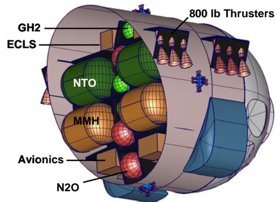
**Figure 10. The terminal landing and ascent propellants are packaged on the back end of the ascender along with external equipment such as ECLSS and some avionics boxes.**
