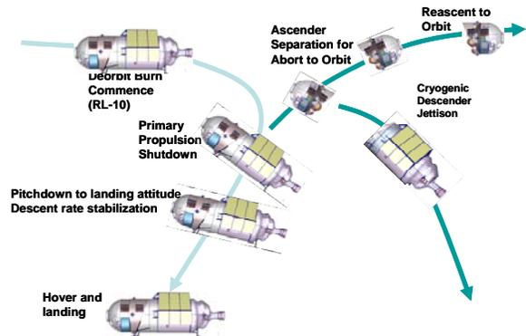
**Figure 7. The proposed design lends itself to efficient nominal landing trajectories, while protecting the ability to accommodate mission aborts.**
