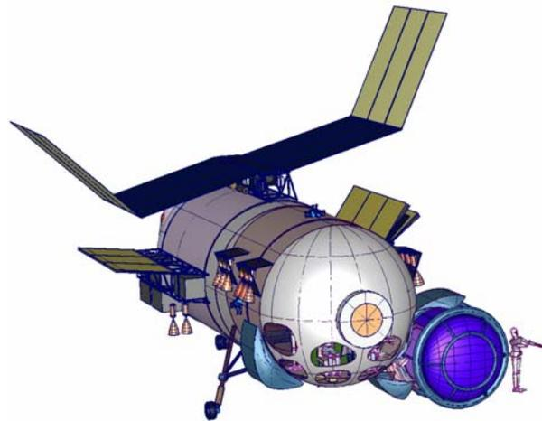
**Figure 11. The solar arrays are designed to gimbal to maximize power even at low sun elevations while also shading the cryogenic propellant tanks and radiators to enhance storage duration and heat dissipation.**
