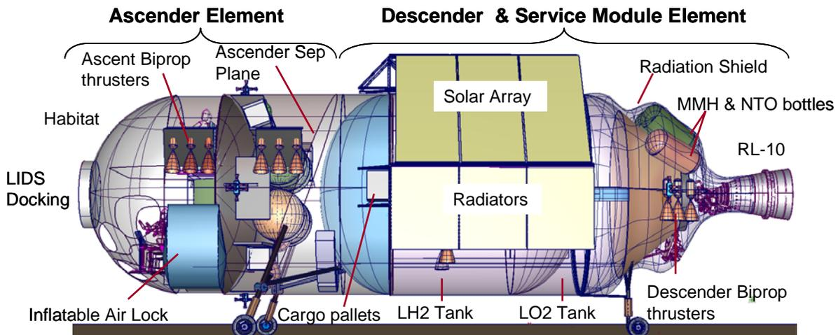
Figure 6. The Dual Thrust Axis lander satisfies the opposing objectives of locating crew and cargo close to the lunar surface with the requirement of large LH<sub>2</sub> tanks and a long, high expansion area nozzle
