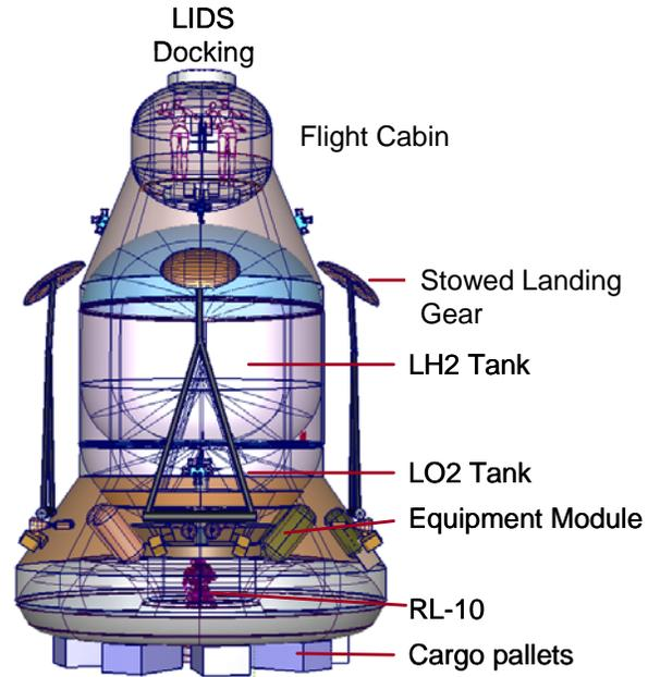
**Figure 15. The Concept 3 Lander has a crew cabin on top, wide, common bulkhead tanks in the middle, and the engine and deployable cargo bay on the bottom.**
