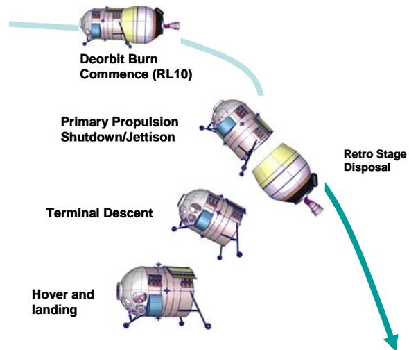
**Figure 12. Concept 2 is similar to Concept 1, but jettisons the large cryogenic propulsion stage following RL10 shutdown, prior to actual landing on the lunar surface in order to minimize the soft landed mass.**
