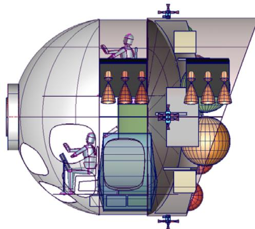
**Figure 8. The Ascender integrates the crew cabin and ascent propulsion into a compact, efficient structure.**
