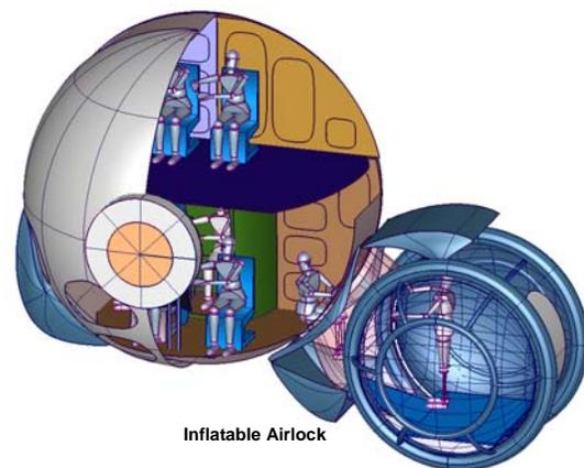
**Figure 9. The crew cabin accommodates four astronauts on the lunar surface and includes a large inflatable airlock at ground level.**
