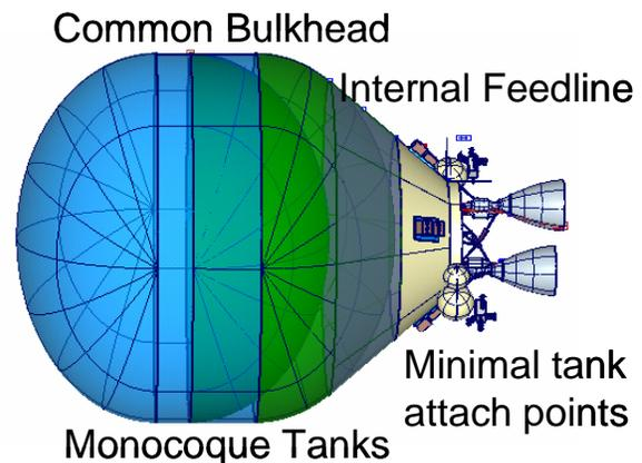
**Figure 5. Using two thin walled monocoque tanks to store the LH<sub>2</sub> and LO<sub>2</sub> propellants results in a very light weight design that efficiently supports orbital cryo fluid management and long duration storage.**
