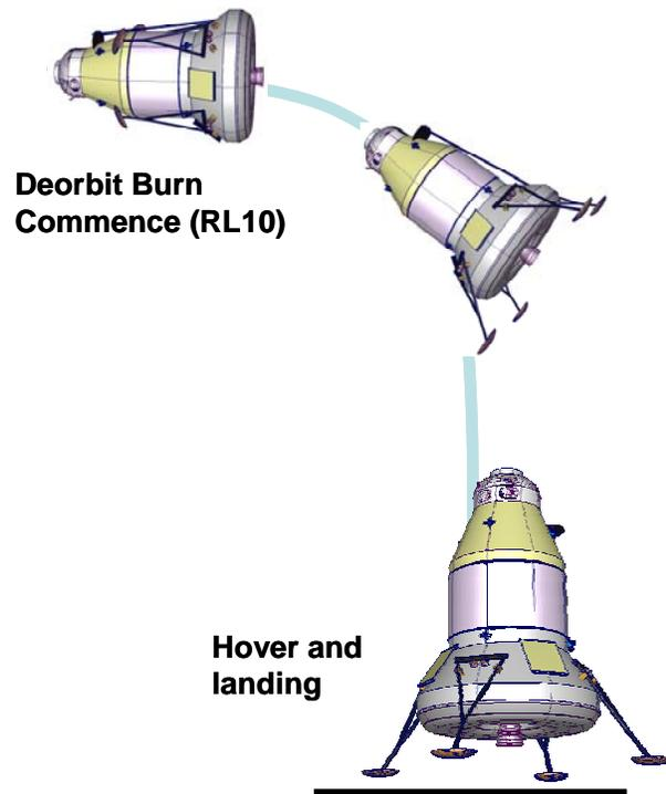
Figure 14. Concept 3 uses deep throttling of the RL10 land on the lunar surface.
