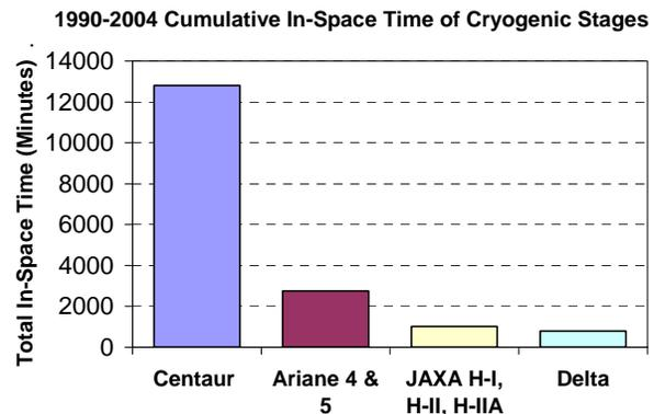
**Figure 2. Centaur's 179 flights over 45 years provide unparalleled cryo-fluid management experience that can guide the design of a cryogenic lander.**
