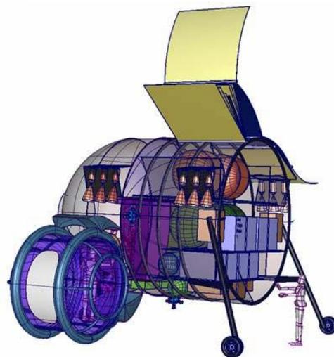
**Figure 13. Concept 2 integrates all of the power, ECLSS and propulsion onto the ascent stage.**
