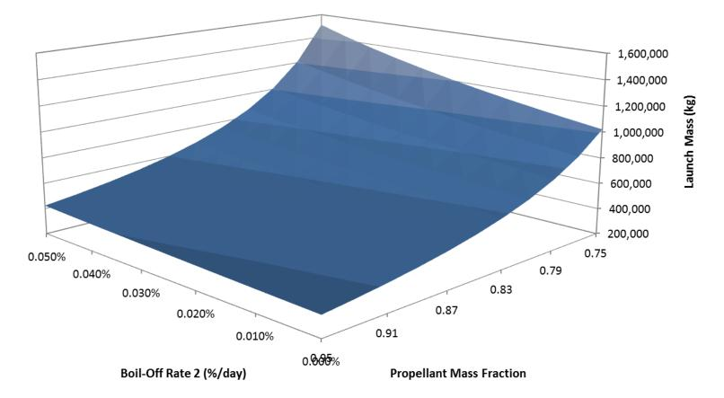
Weak coupling between Boil-Off Rate for CPS 2 and Propellant Mass Fraction
