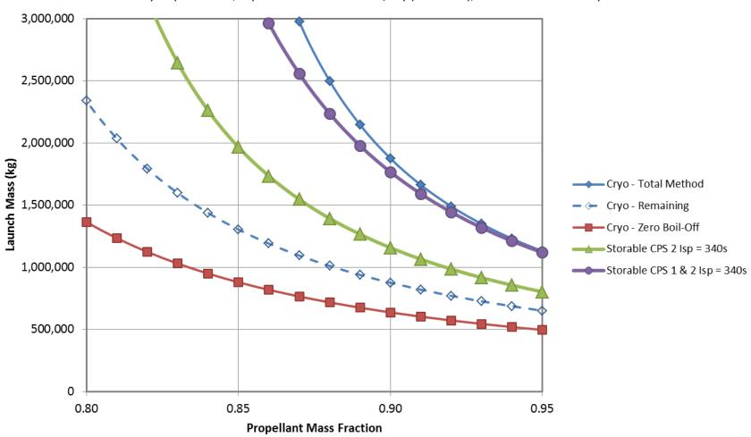
Cryo Isp = 451 sec, Cryo Boil-Off Rate = 0.05%/day (both CPSs), LEO Duration = 180 days
