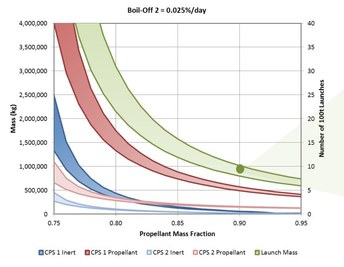
Results for all combinations of design variables with Boil-Off Rate for CPS 2 = 0.025% shown above
